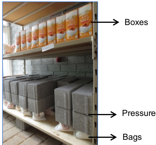
Figure 4: Salt samples and storage condition in a long-term storage test.
